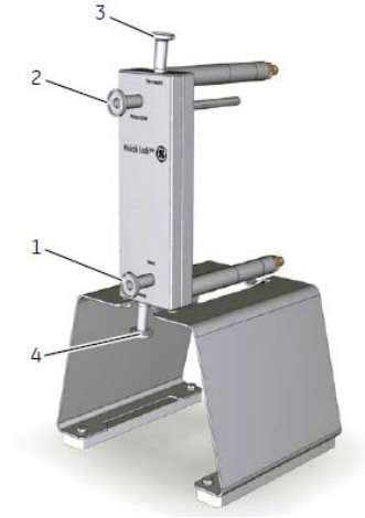
Figure 12. Kwick Lab cassettes and holder II (1) feed inlet, (2) retentate outlet, (3) permeate outlet, (4) permeate port
