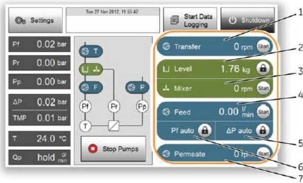
Figure 3. Control panel: (1) Transfer (2) Level (3) Mixer (4) Feed pump (5) ΔP auto (6) Pf auto (7) Permeate
