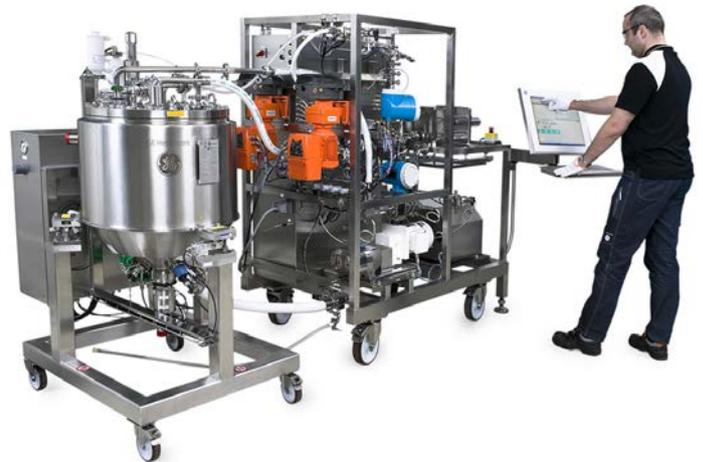
Fig 3. Integrated UniFlux 30 system and 100 L tank allow fully automated CFF via UNICORN system control software.
